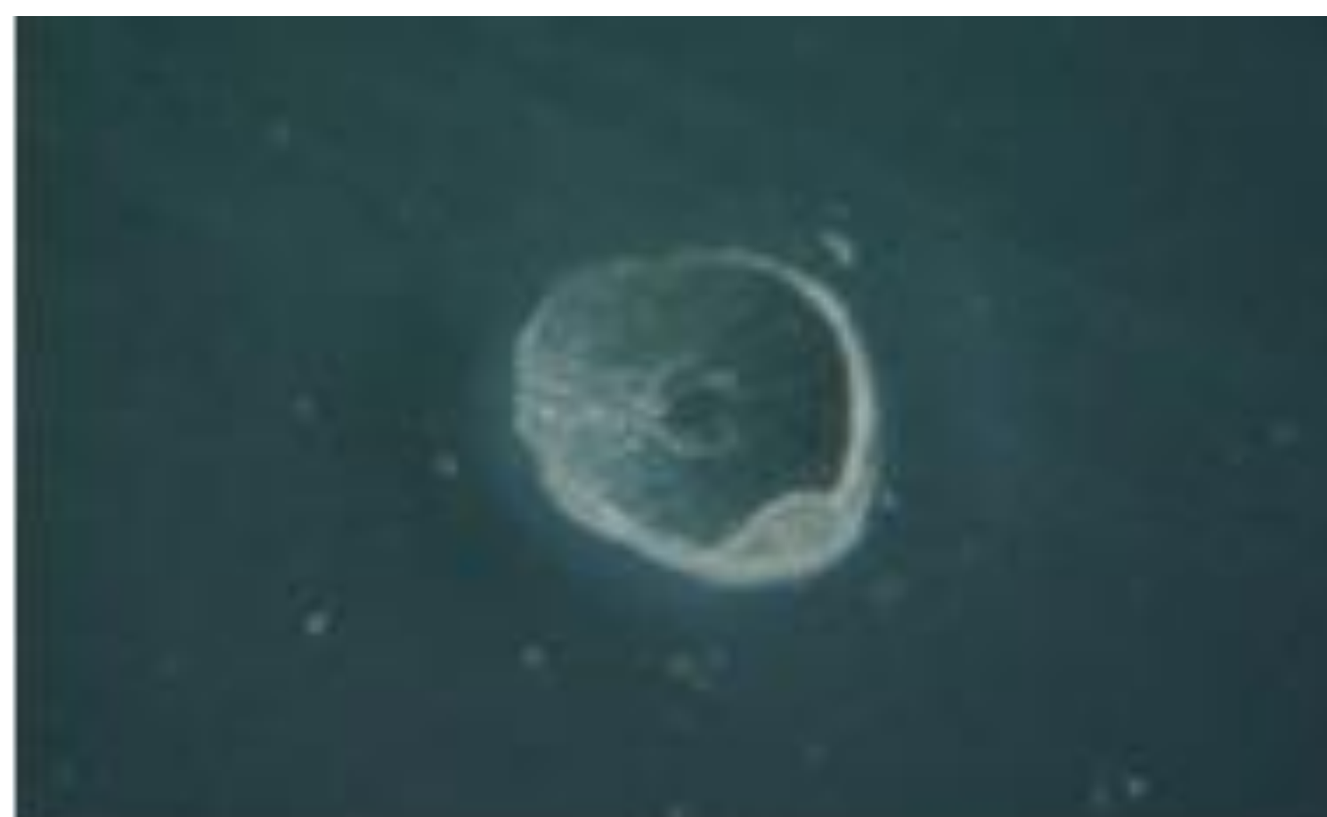
Fig. 1 - PP specimen with defect (void).
