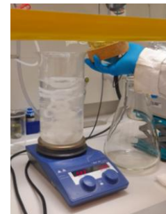
Solvent recovery after filtration
