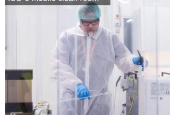
Clean processing inside ISO-6 mobile clean room
