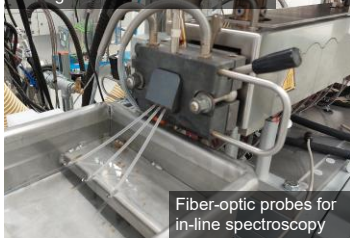
Extruded polymer compound, and cooling in filtered water bath
